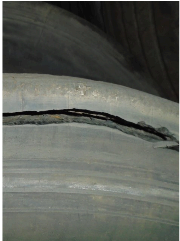
Left: example of a lump in the side of the tyre. Right: example of tyre tread separation.
