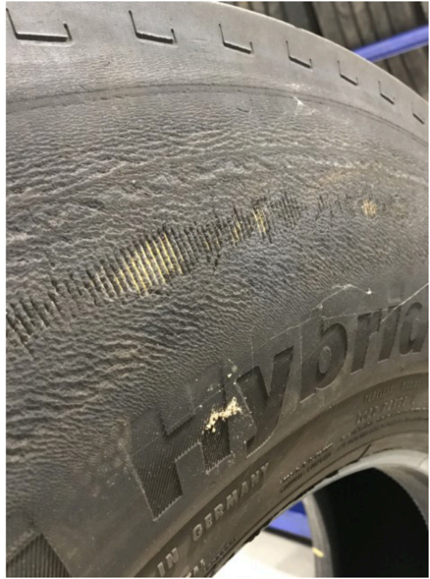
Left: example of a gap in the tyre's tread where the tread depth is less than 1mm. Right: example of visible tyre cord on the side of a tyre.
